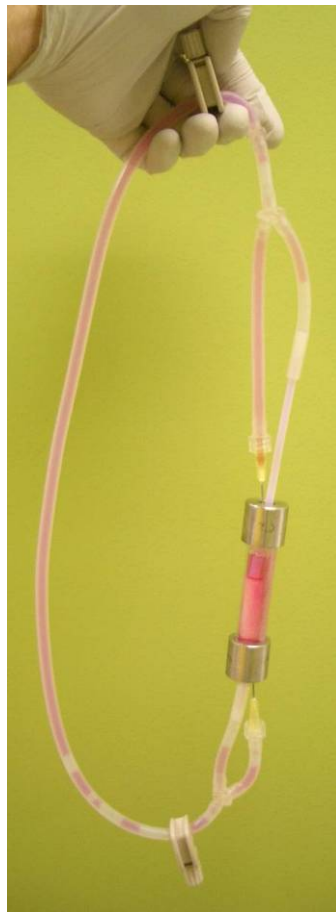
Figure 4.8: Detachable Scaffold-chamber Circuit. The culture chamber and scaffold could be isolated by clamping proximal and distal tubing and closing the ends in an independent circuit while the bioreactor was in a sterile environment, allowing transport through non-sterile environments.
