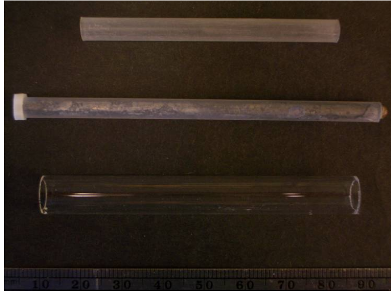
Figure 4.5: Materials for Scaffold Fabrication Using a Glass Tube and a Heat-shrinkable Mandrel. The same mandrel from type III and IV scaffold fabrication was used to fabricate type V scaffolds, but with an outer tubular mold made of glass. The outer tubular glass mold was coated with 1.0% hyaluronic acid and dried overnight. A heat-shrinkable mandrel was placed over PTFE tubing straightened by an internal steel rod and inserted into the outer tubular glass mold. A PTFE ring similar to those used for type IV scaffold fabrication served as a spacer and provided ventilation and alignment at one end of the mandrel. The mold was held vertical with the spacer at the bottom while salt was loaded, fused, and dried into an interconnected salt template. The PTFE tubing and steel rod were slid out through the spacer, leaving the heat-shrinkable mandrel in place. The heat-shrinkable mandrel was removed from the inside of the salt template by heating at 120°C, and the salt template was cooled prior to PGS addition, solvent evaporation, and curing. The outer tubular glass mold and resultant PGS tube were placed in a water bath to dissolve salt. After 24 hours in the water bath the PGS tube moved freely in the outer tubular glass mold and was removed to a second water bath. The PGS tube was sectioned into 30-mm scaffolds and lyophilized. Ruler divisions are 1.0 mm.
