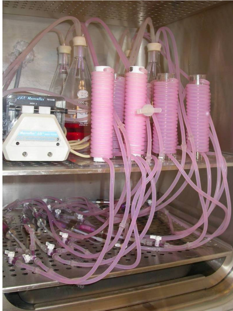
Figure 4.7: First-generation Bioreactor with Pulsatile Perfusion. Reservoirs, gas exchange coils, and the pump head can be seen on the incubator's upper shelf. Scaffolds and chambers were placed below to maximize low-level hydrostatic pressure.
